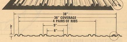
THE BI-RIB SHAPE is a remarkable combination of mechanical strength, attractiveness and economy. BI-RIB can be applied with confidence to all types of farm and industry buildings - as well as a multitude of other applications.
