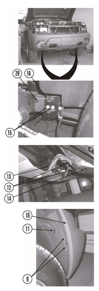
m. Install bracket (13) on shroud (14) with two bolts with captive washers (12).
